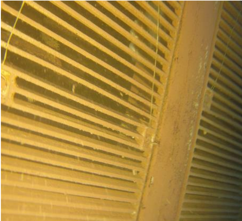
Sea Chest Grids after 15 months protected with HASYTEC DBP
