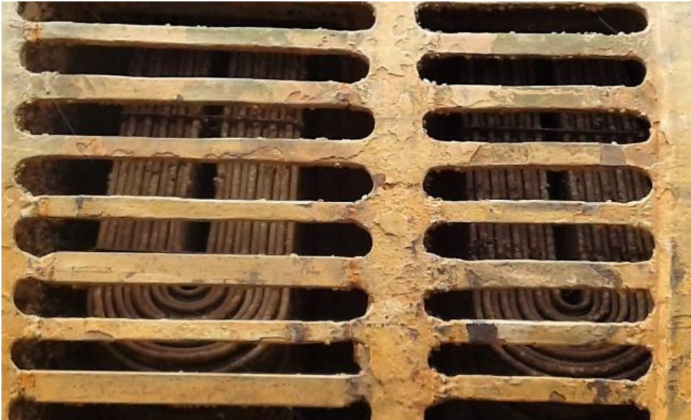
Box coolers & Sea Chest Grids after 12 months protected with HASYTEC DBP
