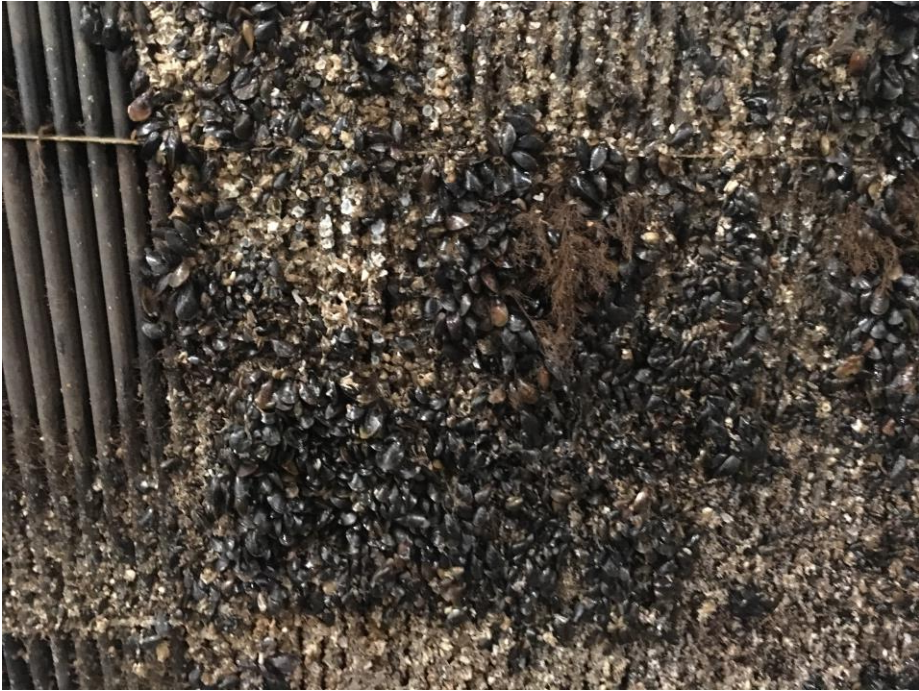
Box cooler after 8 months without HASYTEC DBP
