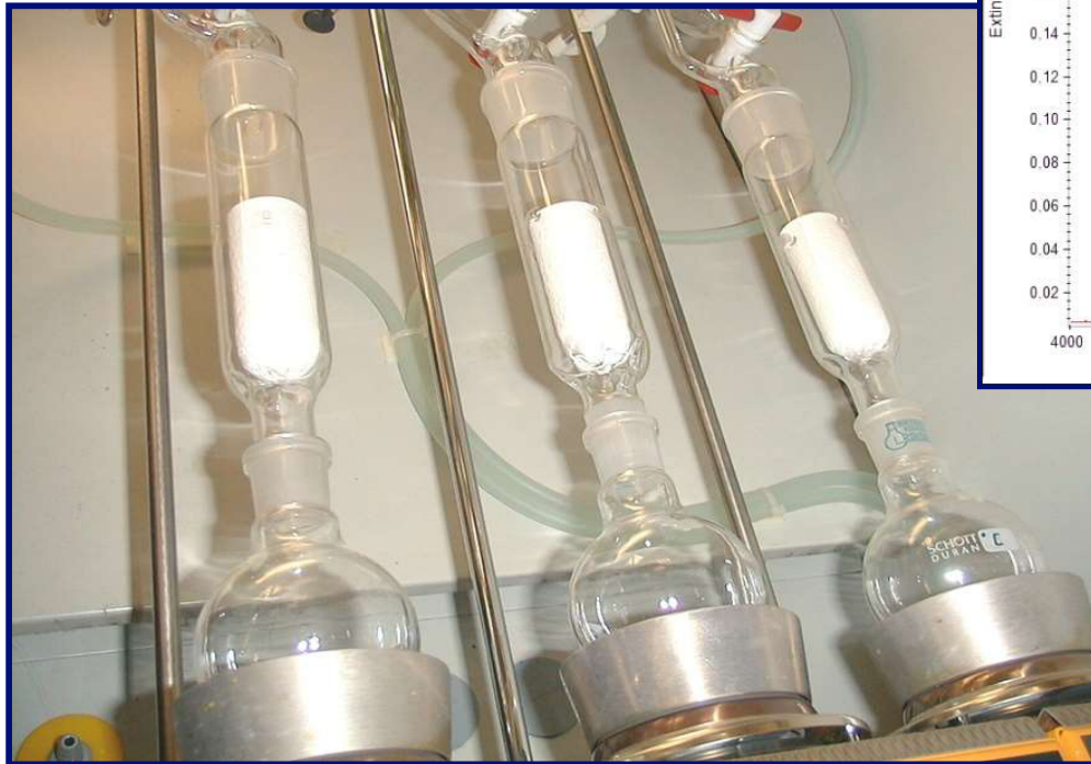
Extraction test equipment
