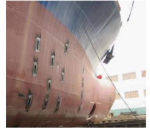
Fig. 13. Side view of the Filia Ariea (84.95 m (Lpp), 13.75 m (Brd), 5.55 m (Dmd), 1440 kW (power)). WAIPs were installed on the ship as shown. (From Murai et al., 2010).
