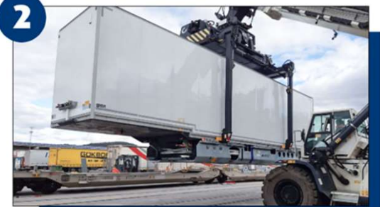
Loading the r2L basket together with the trailer onto a pocket wagon
