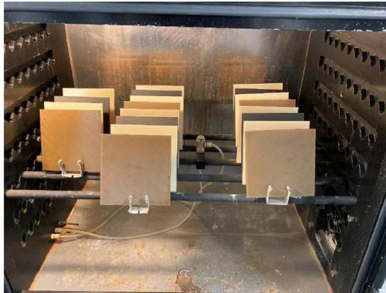
Figure 5: Test set up during Salt Mist
