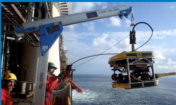
Deploying Remotely Operated Vehicles [ROVs] from offshore oil and gas installations just got considerably easier for repair and maintenance specialists EM&I Alliance – thanks to a REID **TDAVIT** and **PORTABASE** Counterbalance combination.
